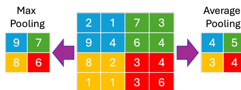
Figure 7.8: Pooling in a CNN. Left: Max Pooling; Right: Average Pooling.
